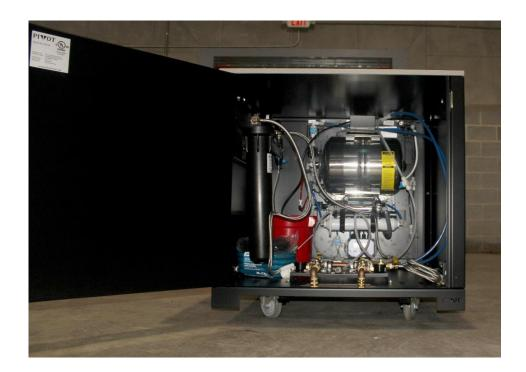
Alternatively, a Water Filtration Cart can be added to this Enhanced Pop-Up Store to provide a Config I or Config III Water Filtration System to the Store. Utilizing this configuration, City Water (hard water) can be terminated to the hose bibb mentioned above.
